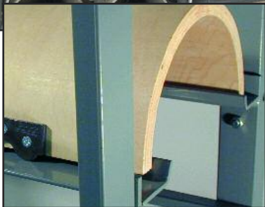
Henderson's exclusive "lip" slide design keeps rotary cutting dies securely centered, preventing damage to the cutting and scoring knives. Numbered racks refer stored dies to customer files or jobs for easy access.
