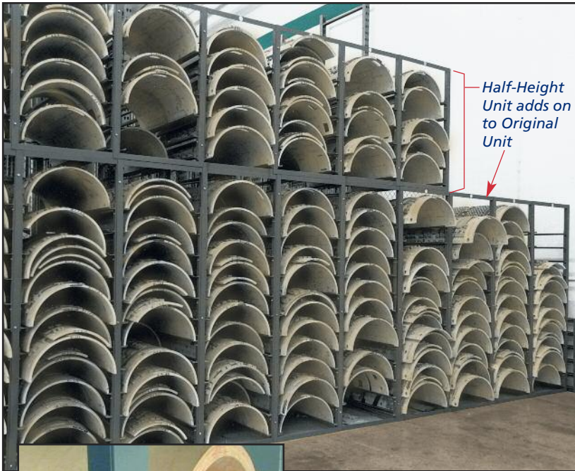
Henderson's exclusive "lip" slide design keeps rotary cutting dies securely centered, preventing damage to the cutting and scoring knives. Numbered racks refer stored dies to customer files or jobs for easy access.
