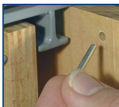
The "T" rack slides used on Platen storage systems. Dies slide in the channels supported by 2 pins.
