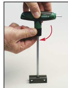
T-handle 6mm Hex Key features a "speed sleeve" for quick sinch-up of loose quoins.
