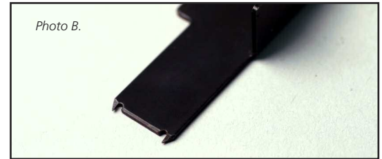
Photo B. A close-up of the 'barbed' end of a Wagner Stripping Claw, these barbs help to securely direct the waste through the female side of the stripping unit, without the need for bottom pins.
