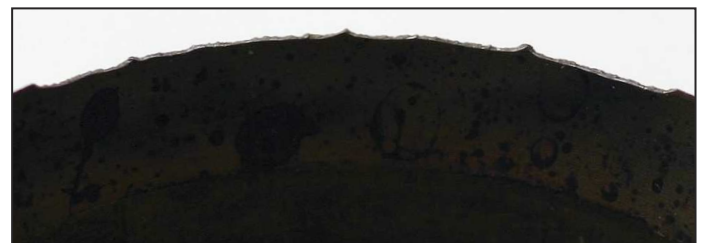
Punch cutting edge damage on a Straight Outside Diameter Punch prompted by uneven mallet blows to edge during insertion into die board.
